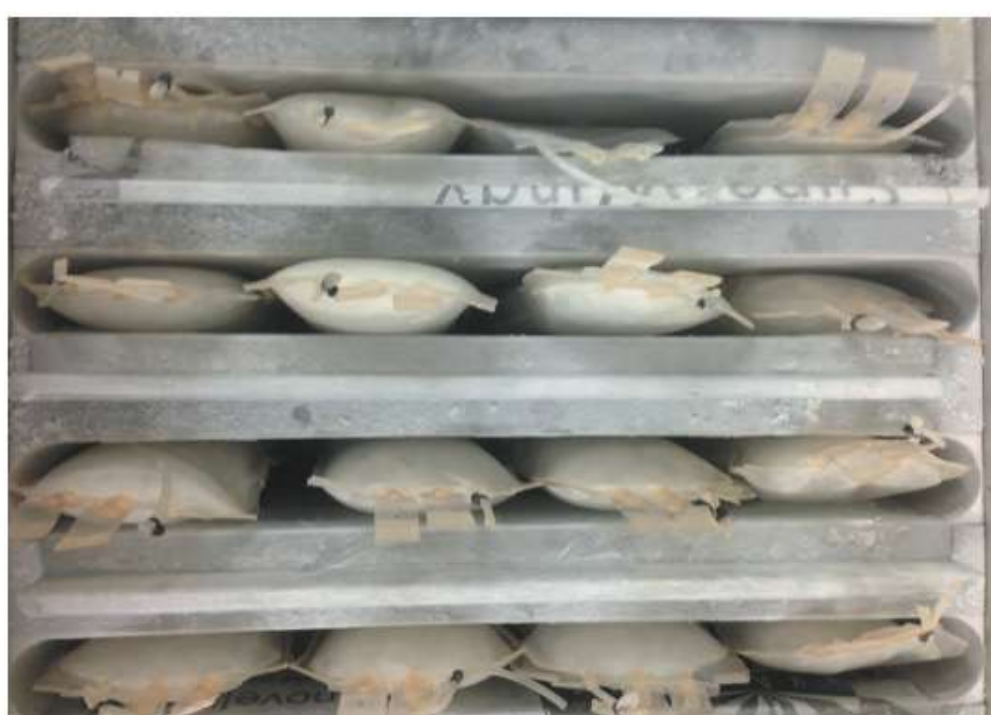
Internal case of the rapid freezer with standard 1000 ml. bags in freezing
